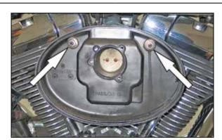
4. Remove the two crank case breather bolts shown.
